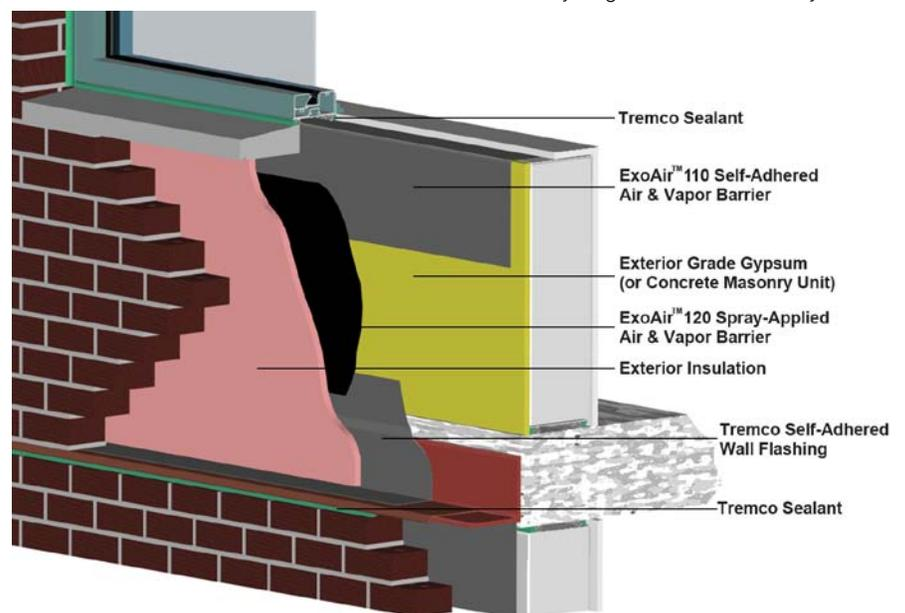
Drying of the wall cavity should be promoted in one or both directions. Air and vapor barriers prevent both air infiltration and vapor diffusion and must be positioned on the warm side of the insulation since air moves from the warm side to the cold side.
